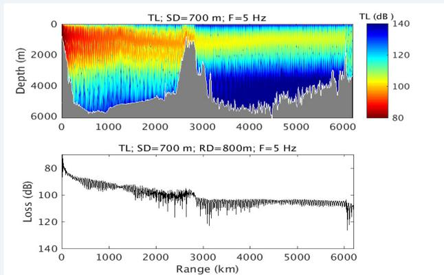
Prediction of sound propagation in the ocean with complex two-dimensional spatial variations in bathymetry and ocean sound speed profiles over a propagation range of more than 6000 km.
